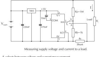
$S_1$  selects between voltage and current measurement. Ra and Rb shown scaled for  $200V_{FSR}$  Rs = 200mV (e.g.  $0.1\Omega/400mW$  for 2A full scale)
