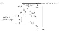
Measuring a 4-20mA loop current.
